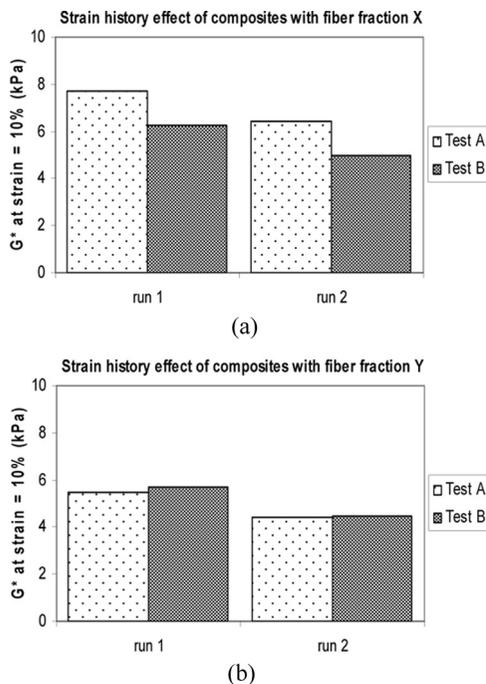
**Figure 3.** Strain history effect of composites containing fiber fraction X (a) and Y (b).
