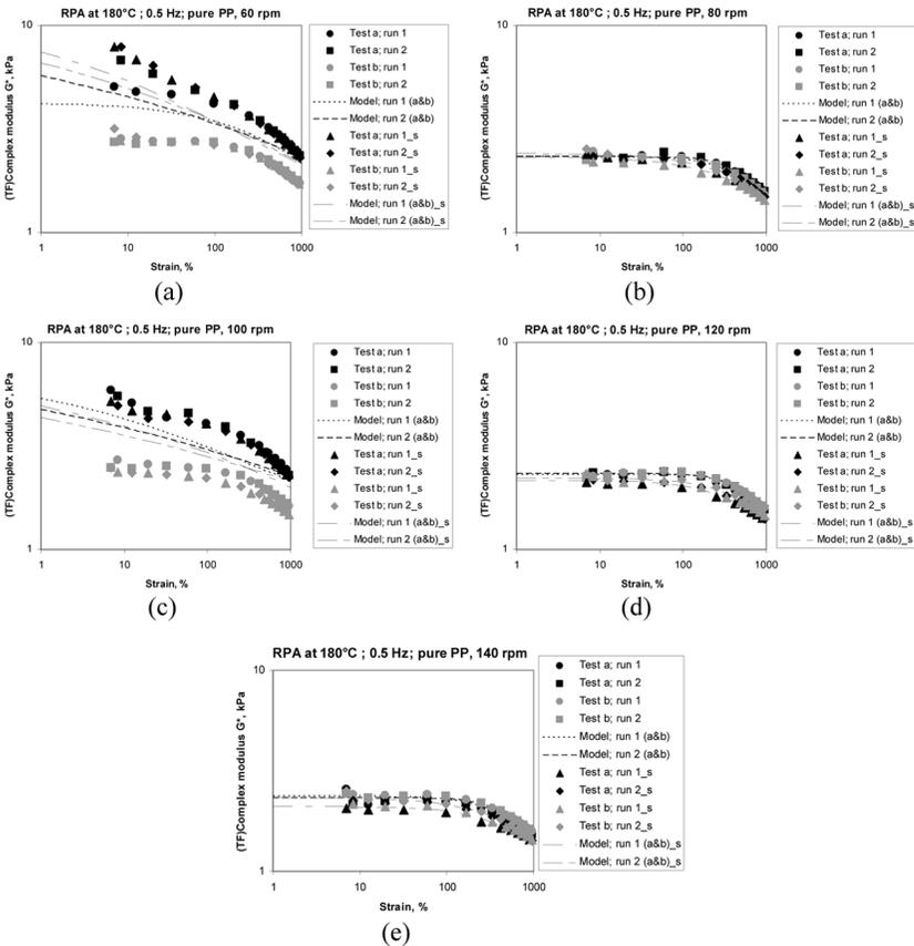
Figure 4. Pure PP at different screw speeds: a, 60 rpm; b, 80 rpm; c, 100 rpm; d, 120 rpm; e, 140 rpm.
