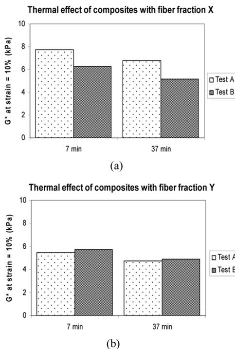
**Figure 5.** Thermal vs. strain effect in composites with fiber fraction X (a) and fraction Y (b).
