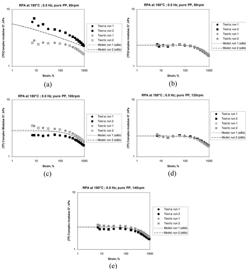
**Figure 1.** Pure polypropylene extruded at different screw speeds: a, 60 rpm; b, 80 rpm; c, 100 rpm; d, 120 rpm; e, 140 rpm.
