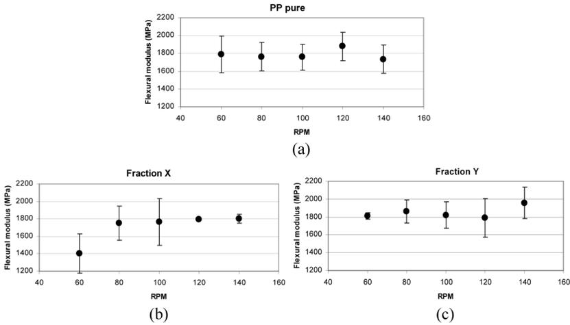
**Figure 6.** Flexural modulus of pure PP (a) and composites with fraction X (b) and fraction Y (c).
